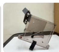
3D printed connecting rod for the MRI alignment indicator
