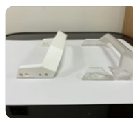
3D printed connecting rod for the MRI alignment indicator
