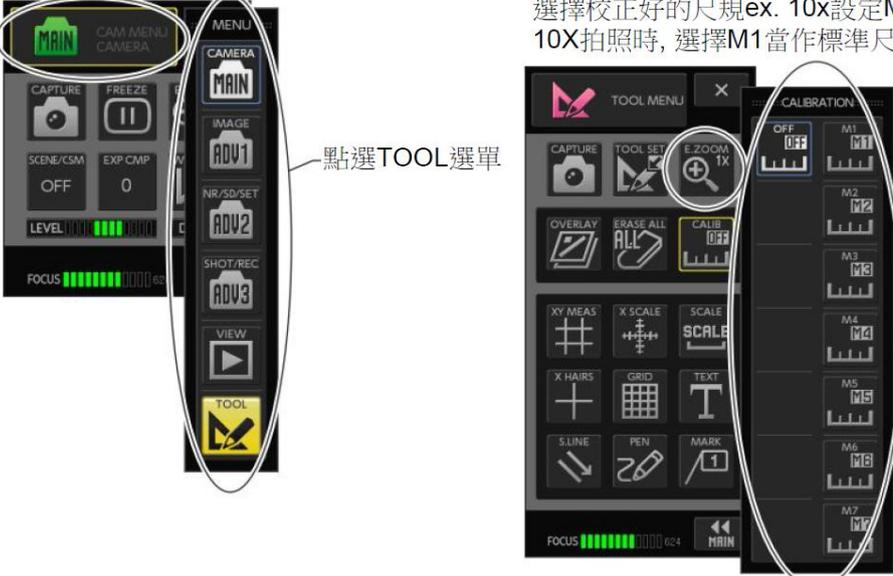
The first screenshot shows the 'CAMERA' menu with the 'TOOL' option circled. The second screenshot shows the 'TOOL MENU' with the 'CALIB' option circled, and the 'CALIBRATION' screen with the 'M1' scale selected.
