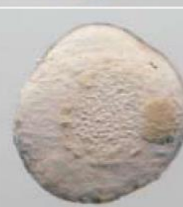
Oblique illumination ("negative" relief contrast)
