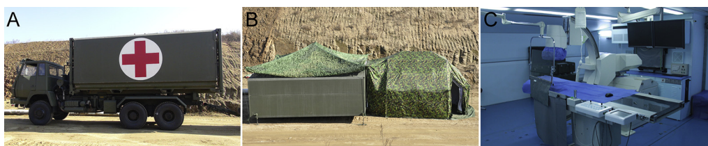
Fig. 2. The field hybrid operating shelter. (A) The shelter in transit. (B) The shelter when seen from outside. (C) The shelter when unfolded from inside.
