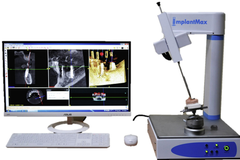
Fig. 2. ImplantMax Workstation as a navigational system on the model.
