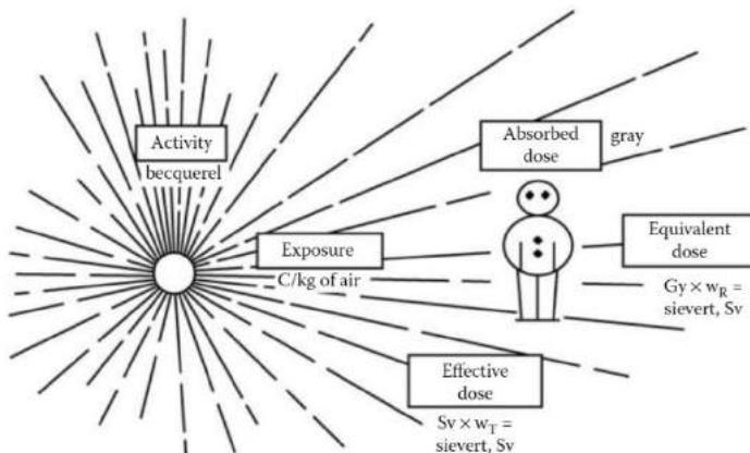
**FIGURE 2.1** The five concepts that relate a radiation worker to a radioactive source: Activity, measured in becquerels; Exposure, measured in C/kg of air; Absorbed dose, measured in grays; Equivalent dose, measured in sieverts; and Effective dose, also measured in sieverts.
