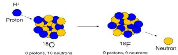
Target Nucleus  $\left( \begin{array}{l} \text{Bombarding} \\ \text{Particle} \end{array}, \begin{array}{l} \text{Product} \\ \text{Emission} \end{array} \right)$  Product Nucleus
