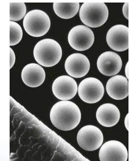
Magnified view of <sup>90</sup>Y glass microspheres (TheraSphere) compared to size of a hair.
