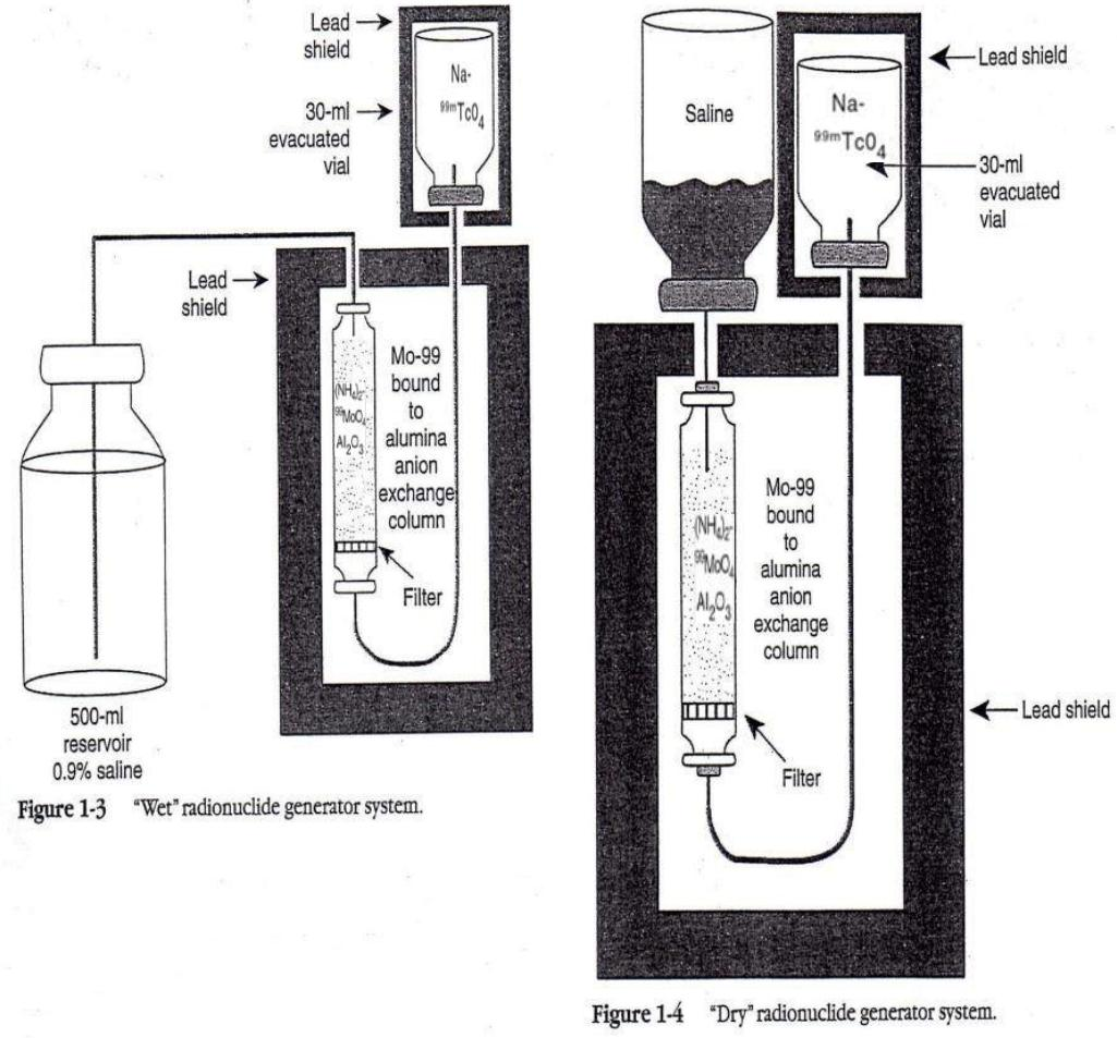
Figure 1-3 "Wet" radionuclide generator system.
