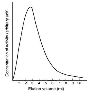
FIGURE 5.4. Elution profile of the  $^{99\text{m}}\text{Tc}$  activity expressed as concentration of radio activity versus eluate volume. The profile may be broader or narrower depending on the type of generator. For generators using fission produced  $^{99}\text{Mo}$ , the eluate volume is about 2.3 ml due to the smaller alumina column.
